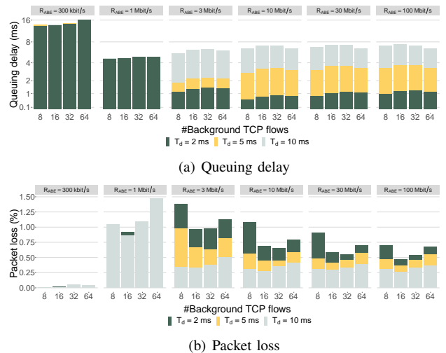
Fig. 11. Queuing delay and packet loss of periodic ABE traffic; ABE traffic rate R_{ABE} , number of TCP flows carried over BE, and delay threshold T_d are varying parameters; other parameters are set as in Table IV.
